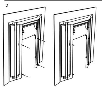
Insert the 4 M6 Studs into the back of the Fireplace Fascia.
