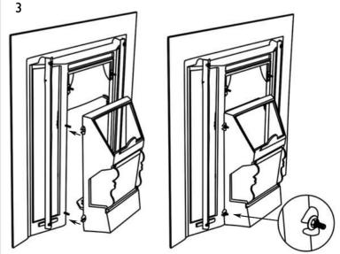
Attach Fireplace Back to the back of the Fireplace Fascia, ensuring that the M6 Studs pass through the fixing brackets on the Fireplace Back. Secure and tighten using 4 M6 Washers and 4 M6 Nuts.
