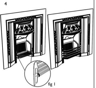
Attach the 2x Fixing Studs into the Bars as shown in fig 1. Slot the now attached Fixing Studs into the holes on the front of the Fireplace Fascia.
