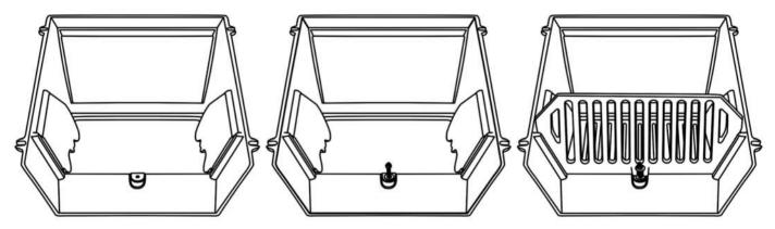
Insert Grate into the groves on the Fireplace Back. Secure and tighten with M6 Nut, M6 Bolt and M6 Washer. THIS STEP IS NOT REQUIRED FOR GAS USAGE. NO GRATE IS REQUIRED FOR GAS USAGE.
