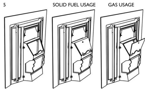
Solid Fuel Usage: Rest the Damper Plate onto the grove on the back of the Fireplace Fascia.
